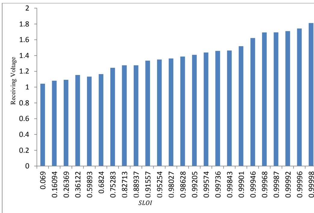
**Figure 4:** Variation of Receiving End Voltage with SLOI
