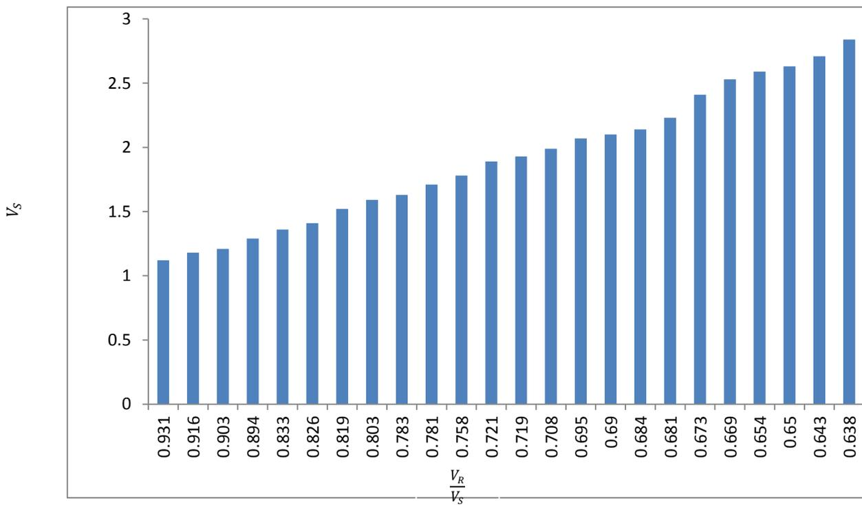
**Figure 8:** Variation of Sending Voltage with Voltage ratio
