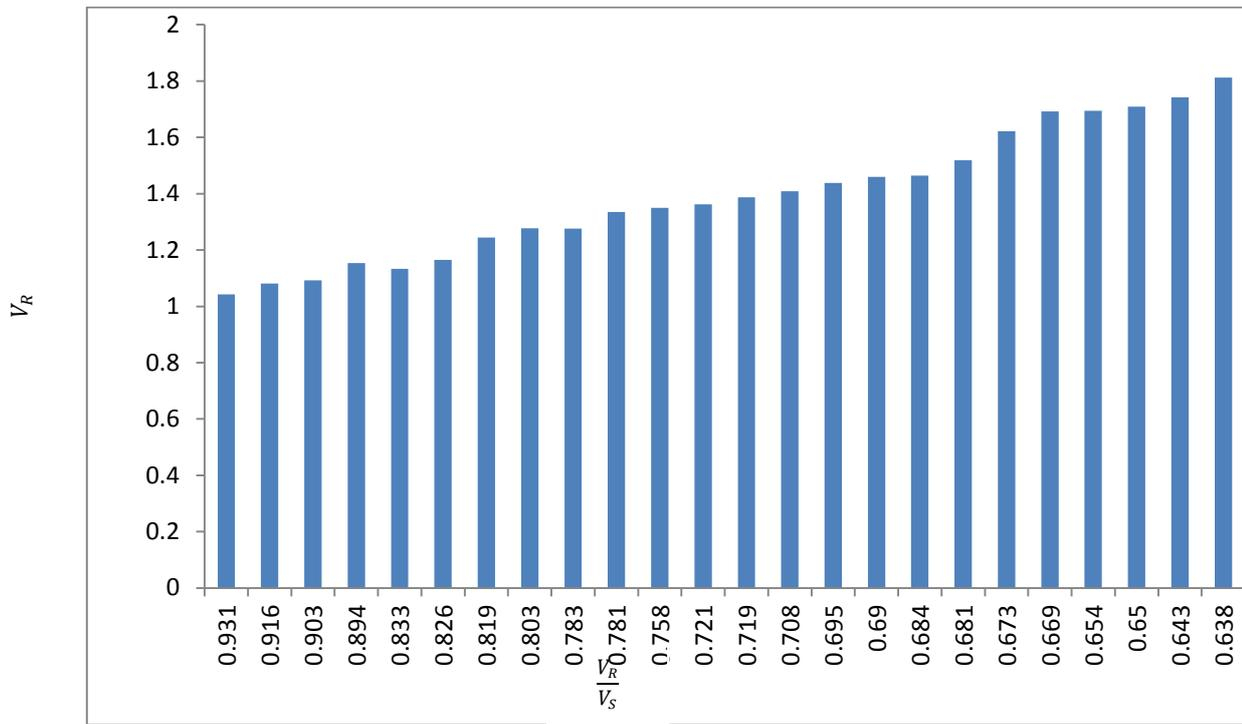
**Figure 7:** Variation of Receiving End Voltage with Voltage ratio
