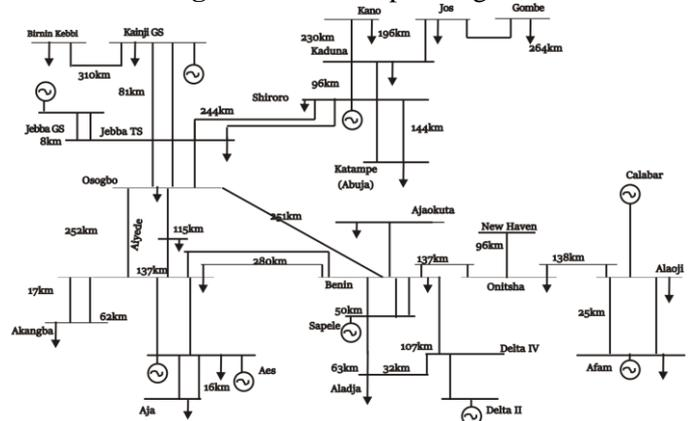
Figure 2: Single line diagram of the Nigerian Power grid
