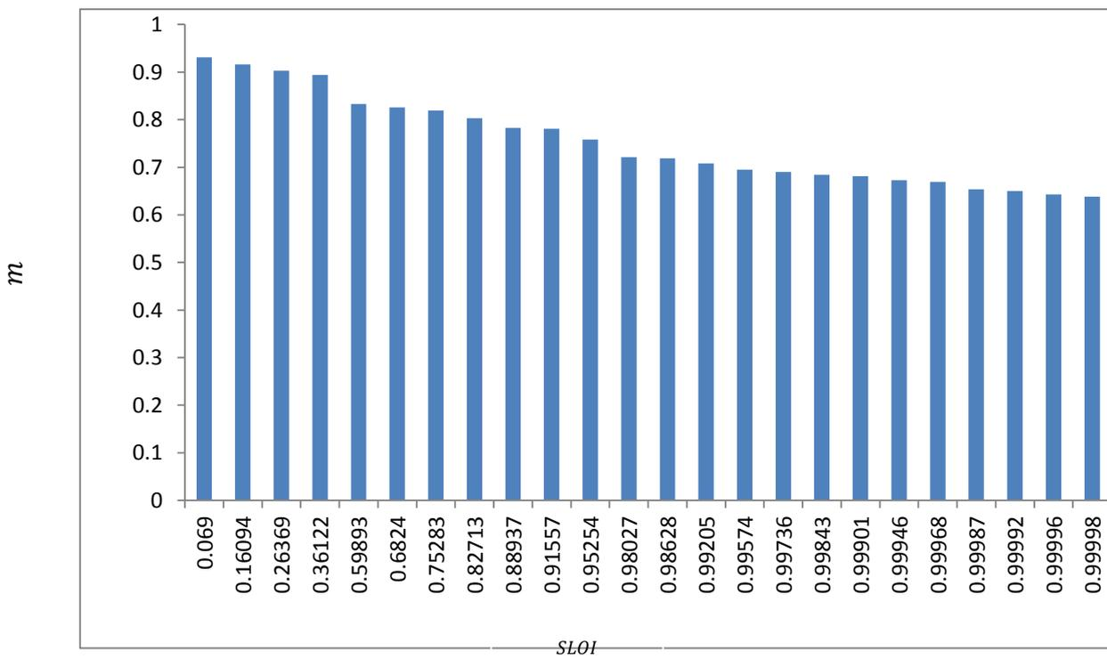
**Figure 6:** Variation of Voltage Ratio with SLOI
