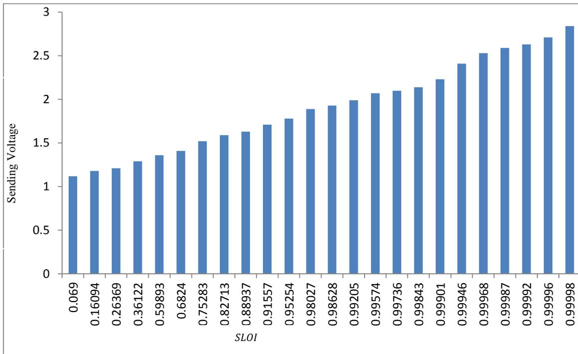
**Figure 5:** Variation of Sending End Voltage with SLOI
