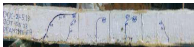
Figure 7. Failure pattern of bottom wrap B1
