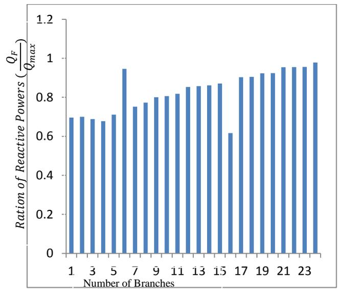
**Figure 17:** Ratios of Reactive Powers versus Branches
