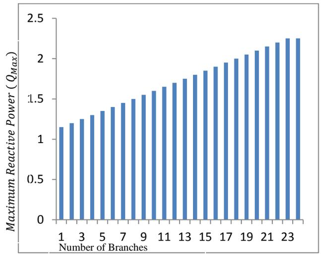
**Figure 16:** Maximum Reactive Power versus Branches
