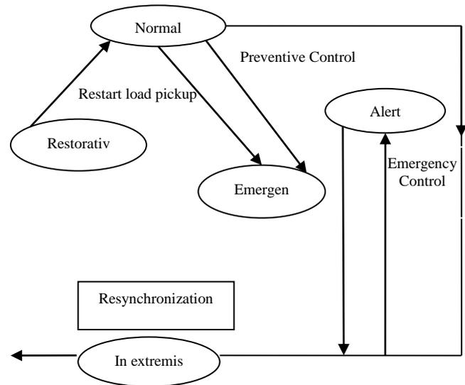
**Figure i:** State Transition Diagram of a Power system
