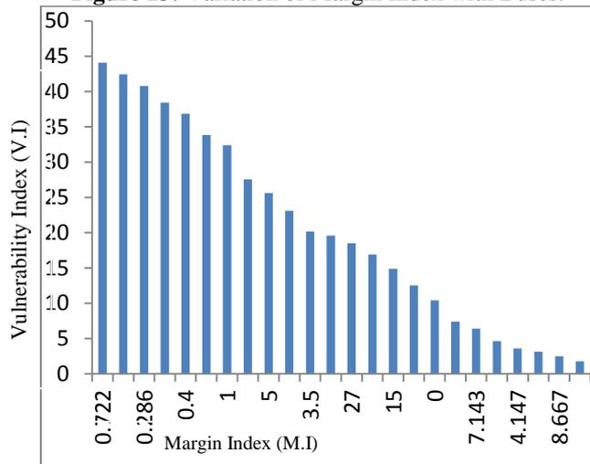
**Figure 14:** Variation of Vulnerability Index with Margin Index.
