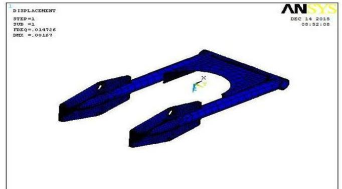
**Figure 9.** Frame Modal analysis of rectangular Suspension Frame
