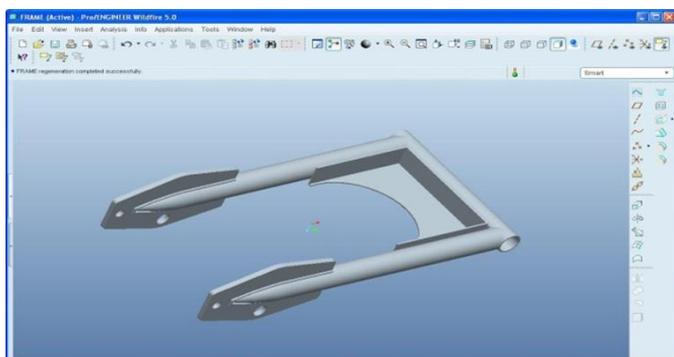
**Figure 7.** 3D model of Rectangular Suspension Frame
