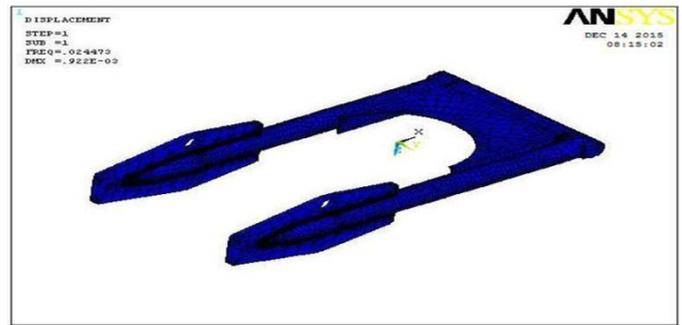
**Figure 8.** Modal analysis of Circular Suspension
