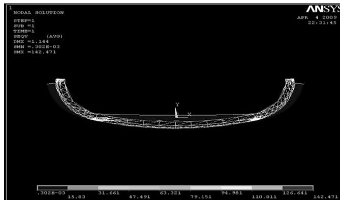
**Figure 5.** Stress Distribution of Composite Bumper
