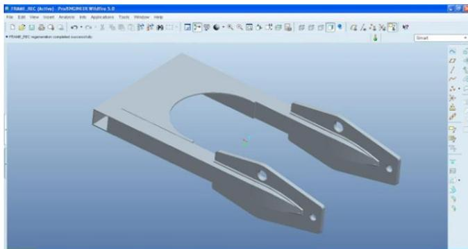
**Figure 6.** 3D model of Circular Suspension Frame
