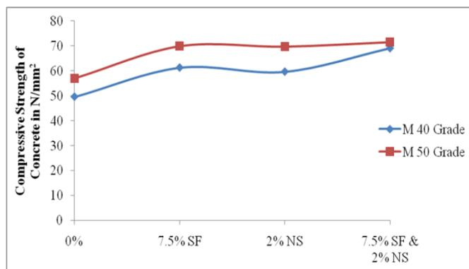
Figure 3.Compressive strength of concrete by using both nanosilica and silica fume
