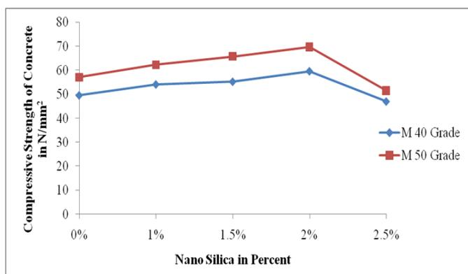
Figure 1.Compressive strength of concrete by using nano silica
