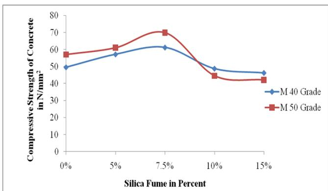
Figure 2. Compressive strength of concrete by using silica fume
