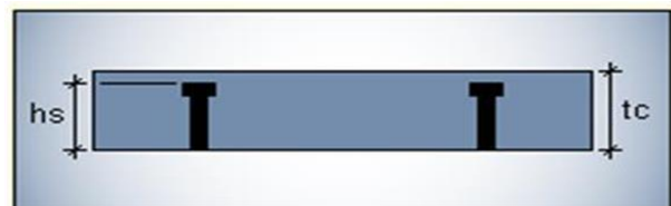
Figure 2.4: Solid Deck Slab
