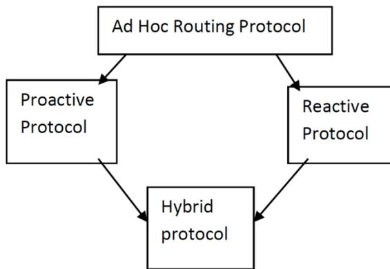
**Figure 2.** Classification of Routing Protocols
