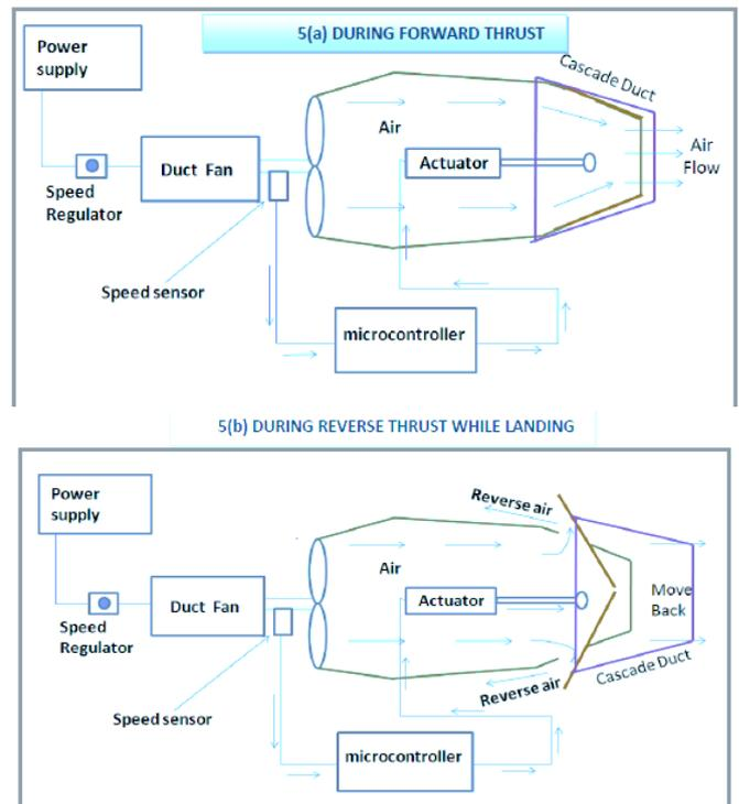
**Figure 5.** Working Principle Hybrid Cascade thrust Reversal Prototype
