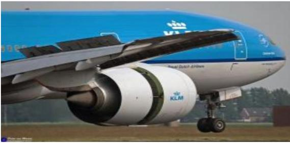
**Figure 1.** Boeing 777 with cascade thrust reverser deployed
