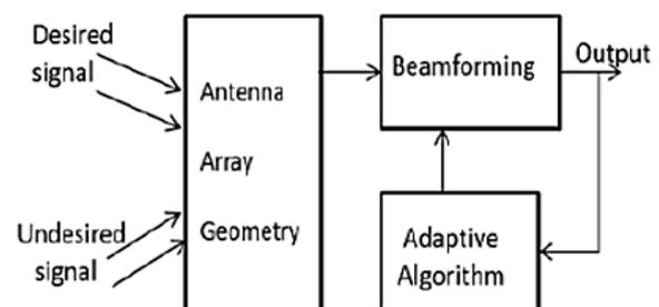
**Figure 1.** Block diagram of Smart antenna system
