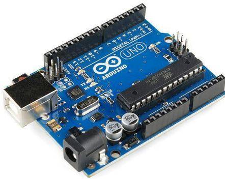
**Figure 3.** Arduino ATMEGA 328 kit
