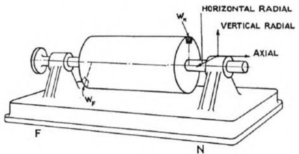
Figure 3: Test rig for dual plane balancing
