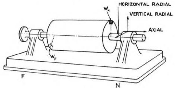
Figure 3: Test rig for dual plane balancing
