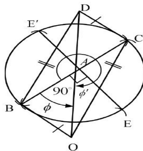
**Figure 1:** A construction procedure for finding the unbalance vector
