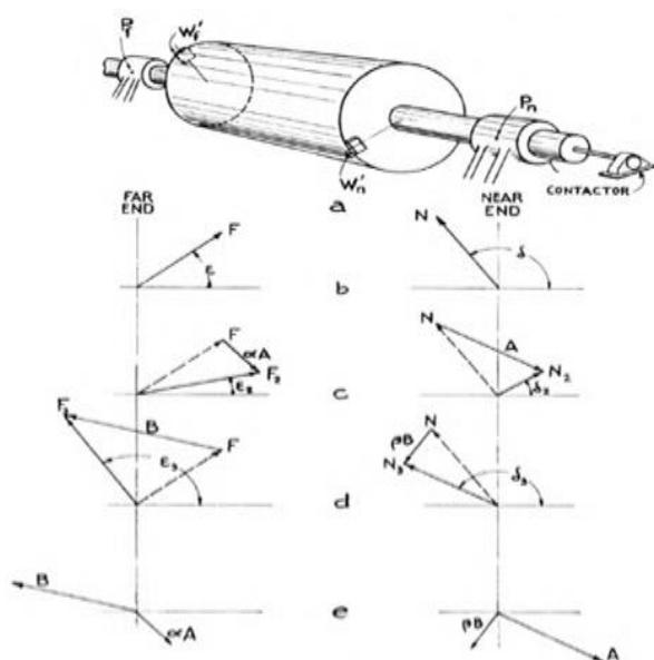
Figure 4: Vector plot in dual plane balancing method
