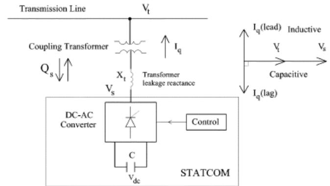
Figure 1. The structure of Static synchronous compensator (STATCOM)
