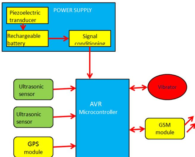
Figure 6. Block diagram of Calciamicus
