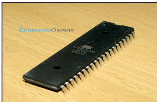
**Figure 2.** Atmega 16 Microcontroller
