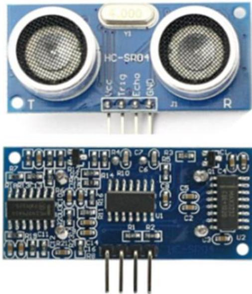
**Figure 2.** Ultrasonic sensors (front and back view)
