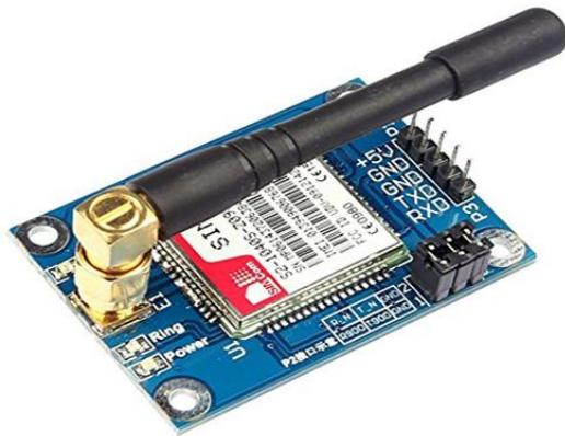
**Figure 3.** GSM Sim 900 Module
