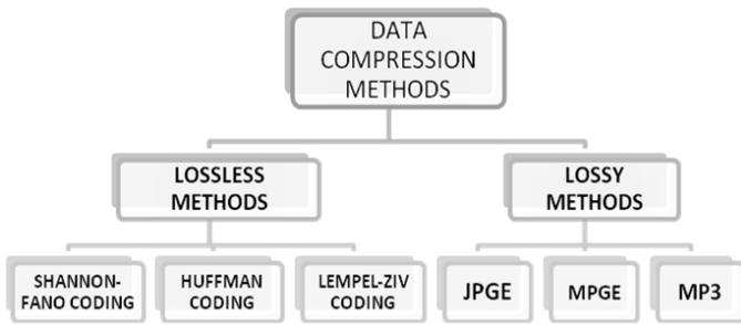
**Figure 1.** Block diagram of Data Compression
