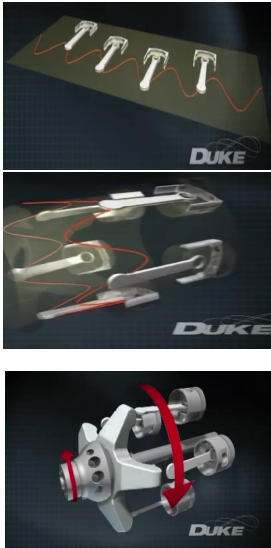
Figure 22. duke engine piston, connecting rod and crankshaft arrangement Sinusoidal motion.
