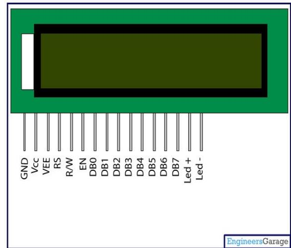
Figure 3. Liquid Crystal Display
