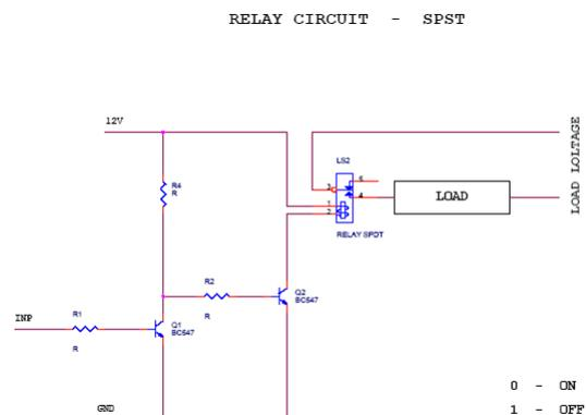
**Figure 6.** Circuit diagram of relay
