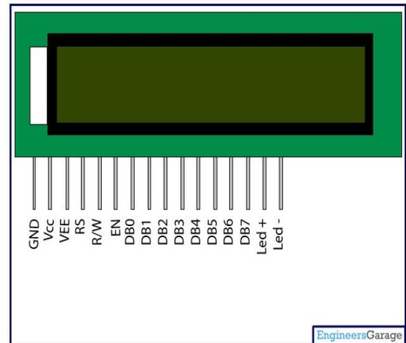
Figure 3. Liquid Crystal Display
