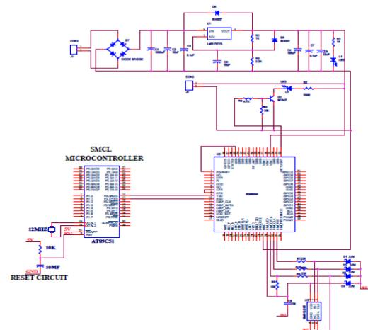
Figure 4. Circuit diagram of GSM
