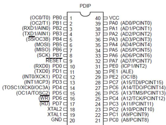
Figure 2. Pin diagram of ATMEGA162V
