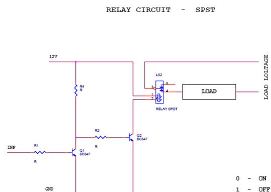
**Figure 6.** Circuit diagram of relay
