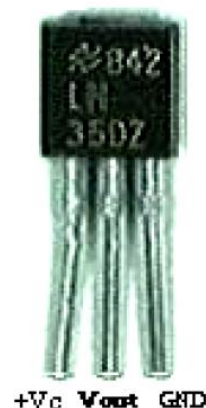
Figure 2. LM35 Temperature sensor
