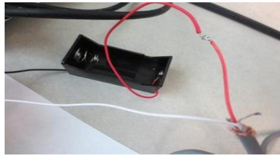
9. Connect the other end of the audio cable to the signal terminal of signal conditioning circuit.
