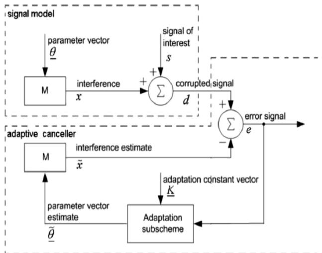
**Figure. 1.** General Structure of Adaptive Interference Canceller
