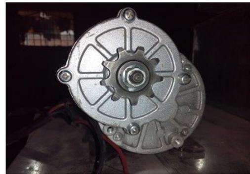
**Figure 2.** DC gear head Motor
