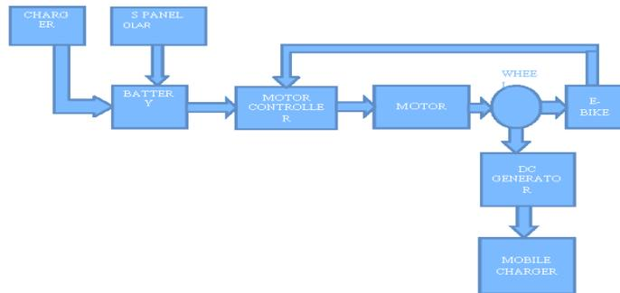
**Figure 1.** Block Diagram of E-BIKE
