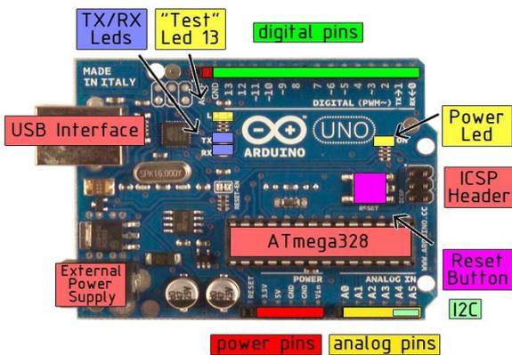
**Figure 5.** Arduino Uno Controller
