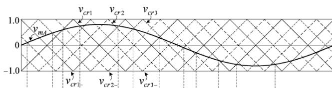
**Figure 4.** Phase shifted sinusoidal PWM modulation.
