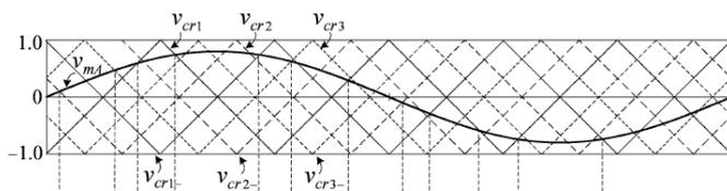
**Figure 4.** Phase shifted sinusoidal PWM modulation.
