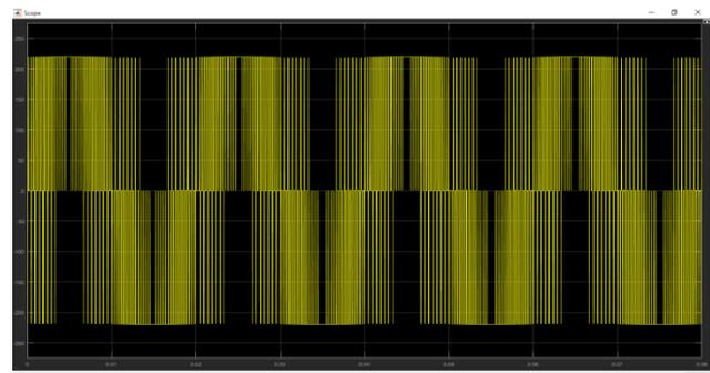
**Figure 7.** waveform of voltage across neutral ( $V_{an}$ )
