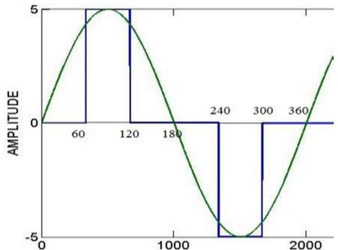
**Figure 2.** Desired pole voltage for three level
