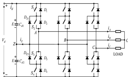
**Figure 1.** Three-level diode clamped inverter
