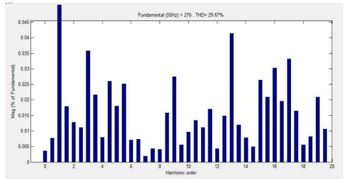
**Figure 2.** Spectrum Analysis of Phase shifted sinusoidal PWM modulation.
