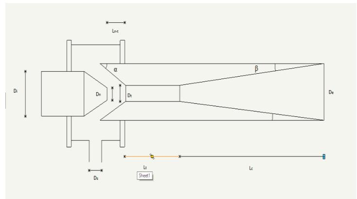
**Figure 1.** Schematically representation of jet pump
