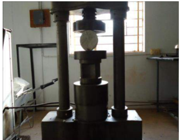
Figure 4 Illustration of compressive strength testing machine with cylindrical shape binary concrete.
