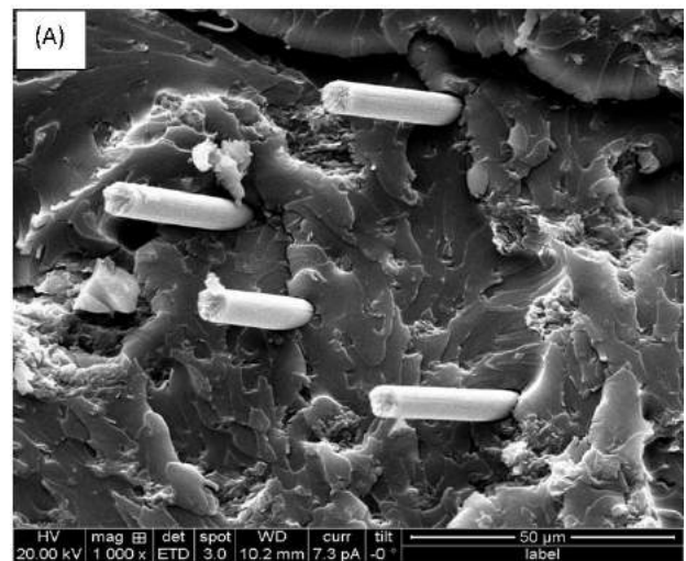
Figure 5: Scanning Electron Microscope Images of (Blend+ Clay )for (a)4wt.% (b) 5% wt.% and (c) 6wt.% blended Nanocomposites as a Function of Clay Loading.
