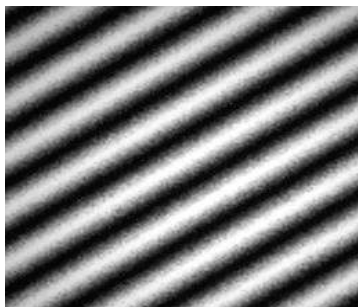
Figure 9: Real fringes of the hard drive enclosure
