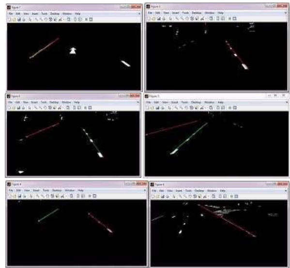
Figure 8. Lane detection results by Hough transform
