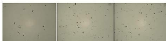
Fig. 4a. Typical CR-39 track detectors seen in the present work for chemistry department.
