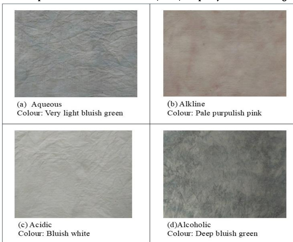
Figure 2. Colours developed on cotton fabric from IC-B (saline) sample dye extraction using different solvents
