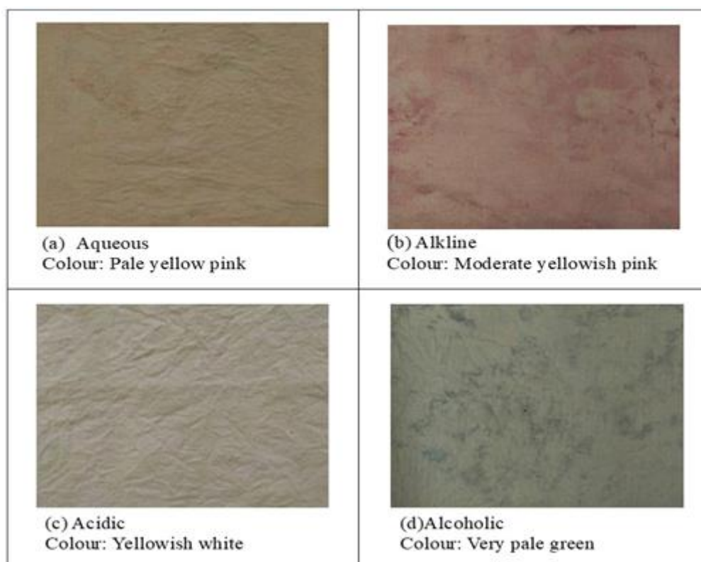
Figure 1. Colours developed on cotton fabric from IC-A (non-saline) sample dye extraction using different solvents
