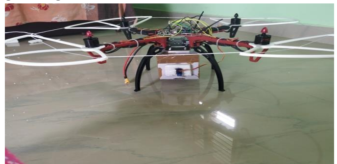
Fig 5: Final Arduino Uno based fire fighter drone dropping mechanism
