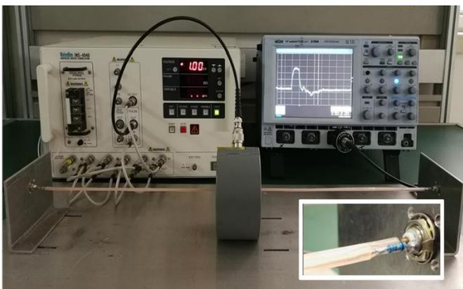
Figure 7: Test setups deployed to experimentally investigate PCI on the case of a straight wire-pair cable
