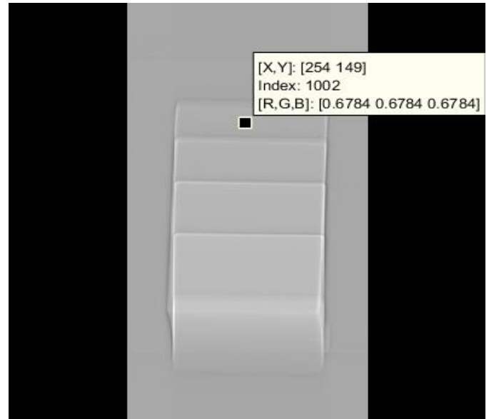
Figure 4. The identification of pixel value on step-wedge phantom images.
