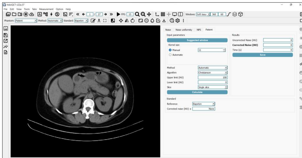
Figure 1. GUI for automated noise measurements using three different methods.
