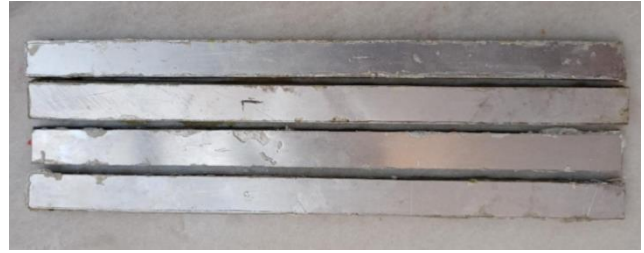
Figure 2: Tensile specimen cut from GLARE
