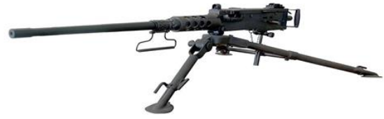
Fig: 4 A .50 caliber M2 machine gun John Browning's design
