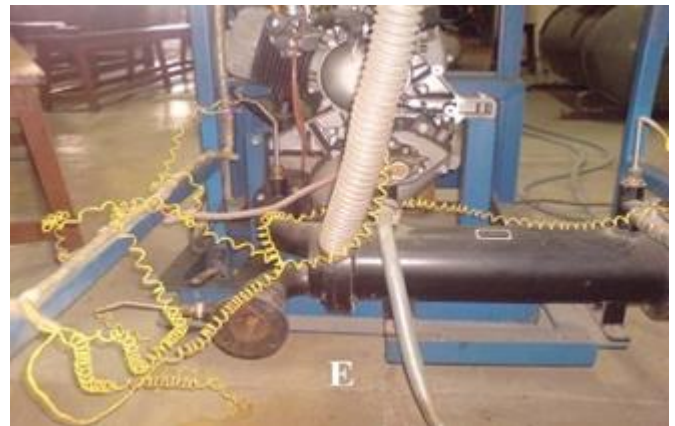
Fig.3.2.3 Location of Exhaust point, "E"
