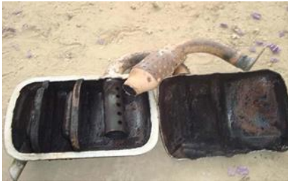
Fig.2.4 Hybrid muffler in cut condition
