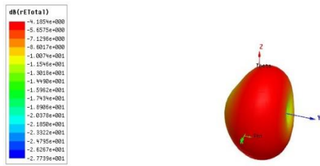
Figure 6 : total rE of the antenna.
