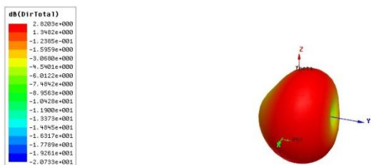
Figure 9 : total Dir of the antenna.
