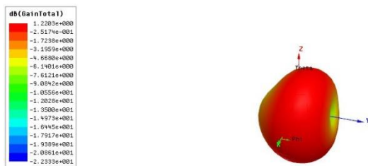
Figure 8 : total gain of the antenna.
