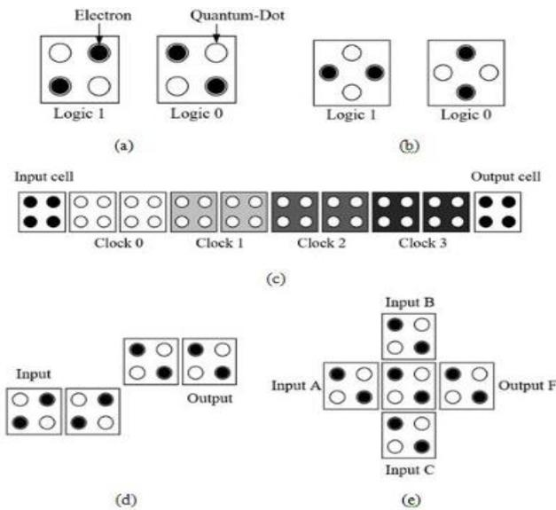
Figure 1 : QCA logic and fundamental QCA components: (a) normal cell; (b) rotated cell; (c) QCA wire; (d) Inverter gate; (e) 3-input majority gate
