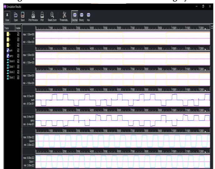
Figure 6: Simulation results for the full adder circuit
