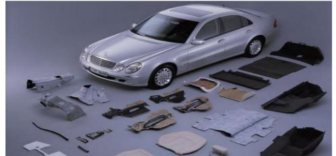
Figure 3. Mercedes E-class automotive components are made from different bio-fiber reinforced composites (Holbery et al., 2013).
