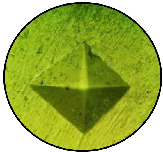
Fig. (4) The indenter of hardness test.
