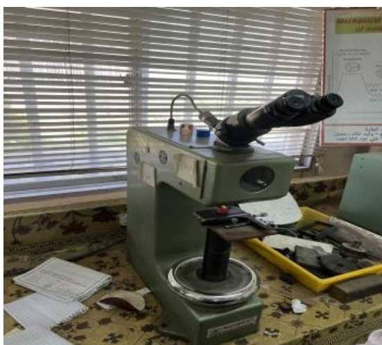
Fig. (3) WOLPERT gadget of type (V-Testor 2)
