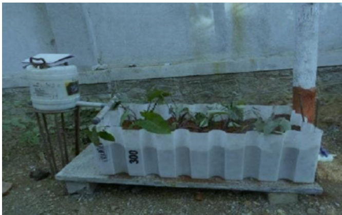
Fig 6 : Pilot model of reactor with Phragmite austrails
