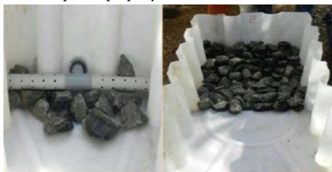
Fig 1: First layer of 40 mm aggregate
