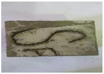
Figure 2. Variation in Geopolymers cement with firing at 900 C0
