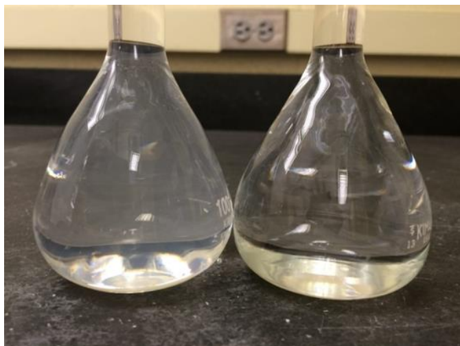
Figure 1 : Precautions to be take while preparing silver nitrate solution- (A) Turbid and white colour solution (B) clear and colourless solution.
