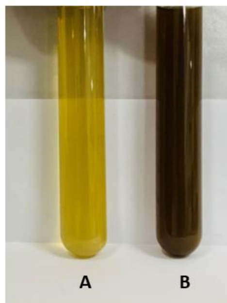
Figure 4: silver nanoparticle synthesis (A) before 24 hours (B) after 24 hours. Colour change from pale yellow to brown indicates the presence of silver nanoparticles.
