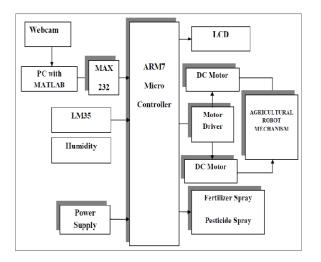
Figure 1: Block diagram of Farming robot
