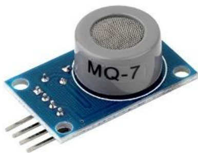
Figure 2. MQ-7 gas sensor module.
