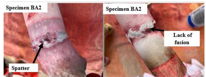
Figure 8 Spatter and Lack of fusion defect after the dye penetrant inspection
