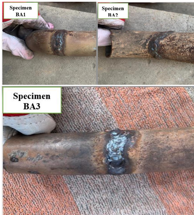
Figure 5 Visual Inspection Result of Butt Joints of the Exhaust Pipes Welded at Workshop
