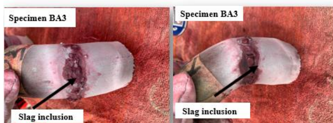
Figure 9 Slag inclusion defect after the dye penetrant inspection
