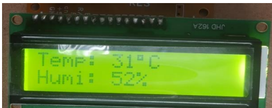
Fig 3. Temperature and humidty values are there by DHT11 sensor and those are displayed on LCD
