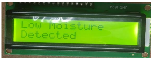
Fig 2. Low moisture which means soil moisture sensor is dry and that result is displayed on LCD
