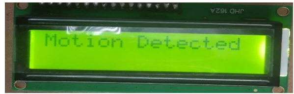
Fig 4. Motion dedetcted through PIR Sensor and that is shown on LCD
