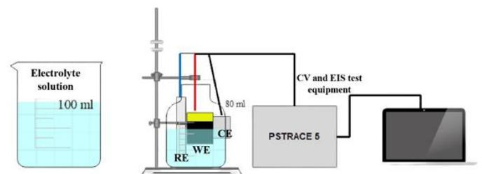
Figure 3: CV and EIS Characterization Techniques
