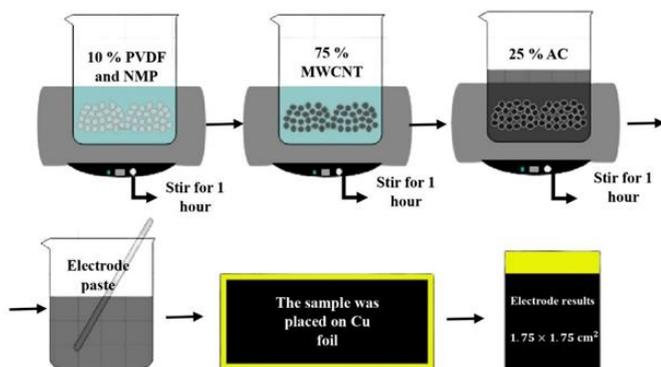
Figure 2: MWCNT/AC Electrode Synthesis
