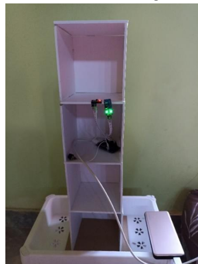
Figure 9: Vibration data acquisition with massage gun
