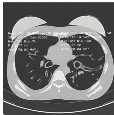
Fig 2. Region of interest (ROI) position for image quality analysis on a breast phantom with a cross-sectional area of 70.04 mm 2
