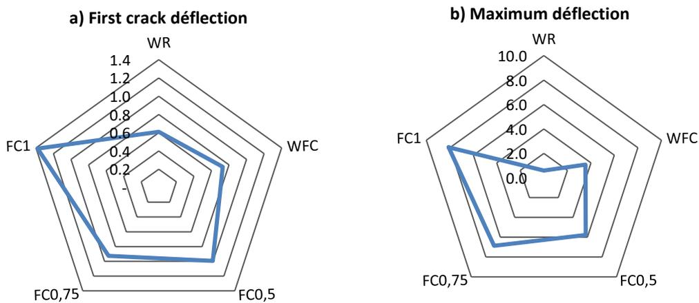
Figure 7. Flexural test results of TRC plates in terms of deflection radars:
