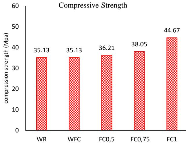
Figure4. Histograms of 28-day compressive strengths.
