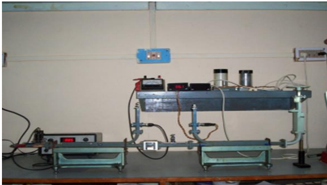
Figure 1 : Microwave Measurement X - Band setup.
