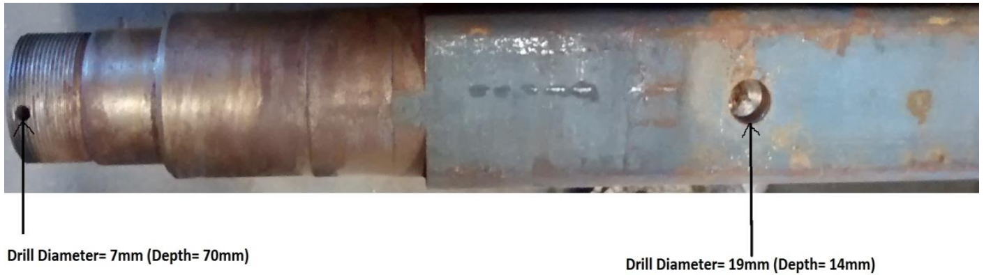
Fig 2: Axle with two drill holes.
