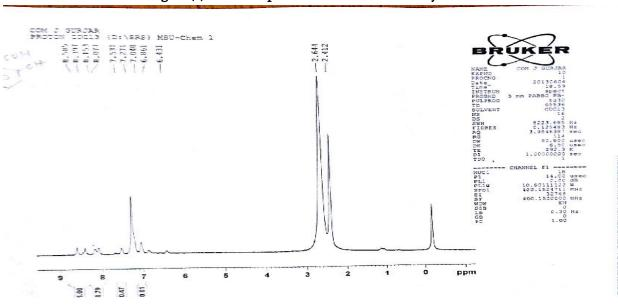
Fig: 1 (a) <sup>1</sup>HNMR Spectrum of m – amino salicylic acid
